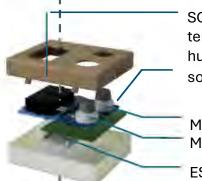
SCD30 sensor – air temperature, relative humidity, CO2 conc soldered PCB
